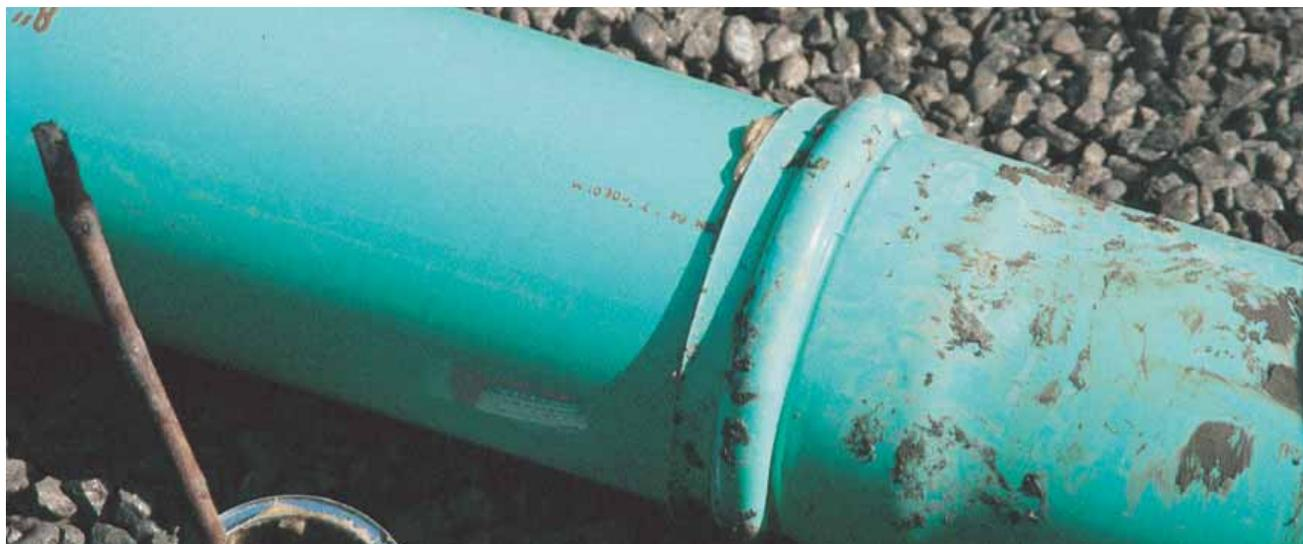
**City of Edmonton 'PVC Pipe Study'** – A comprehensive performance study of PVC pipe installed in Edmonton since 1977 concluded that its service life could be conservatively rated at 88 years or more.
