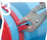
Secure the Pipe Stop using a pair of vice grips.
