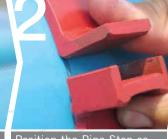
Position the Pipe Stop so that it just covers the insertion line.
