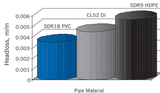
The 'C' factors obviously have a significant effect on flow rates. Comparing various materials it can be seen that PVC pipe has a much lower headloss at any given flow than other common piping materials.
