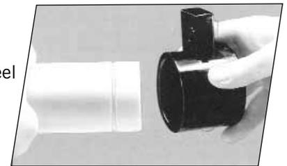
Any material left as a feather edge in the groove should be removed. Care should be taken not to damage the square edge (shoulder) of the groove, particularly at the edge near the spigot end of the pipe as this is the primary sealing surface. Feathered or rounded edges, may indicate a worn tool and may result in possible leakage. Make sure the grooved shoulders are sharp.
