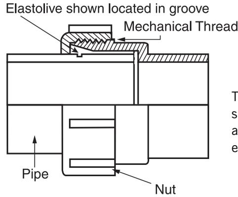
The 3" and 4" joint design differ from smaller versions in that the sealing ridges are located on the fitting and the elastolive extends to the end of the pipe.
