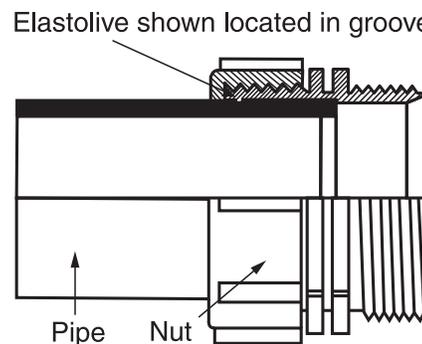
Once engaged in the groove, the elastolive virtually becomes part of the pipe and when the nut is tightened, the pipe is locked into the fitting.
